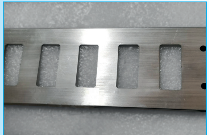
Calibration stencil for the realisation of high-precision strip / slit strip width measurement
